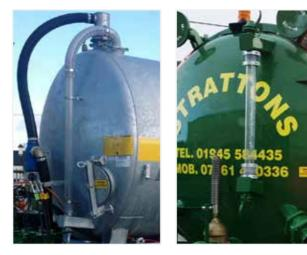
Full Length Sight Tubes: To allow the operator to easily identify how much liquid remains in the tank.
