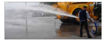
Washdown Hose Assembly: Consists of a 2" gate valve and 2" quick hose connector
