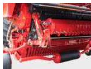
Additional tracking roller for pick-up
