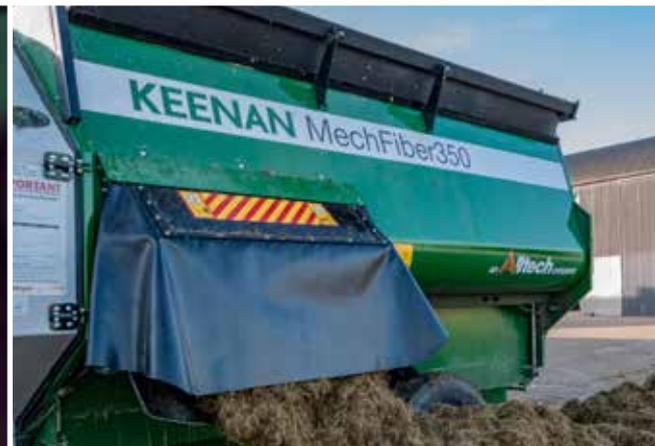
The design of the KEENAN MechFiber350 makes it the perfect mid-range machine for incorporating high levels of dense fibrous material into diets. The wide mixing chamber creates more space for the gentle tumbling action that produces the KEENAN MechFiber ration consistently. This high volume machine is capable of discharging feed over barriers 1,346mm (53") high.
