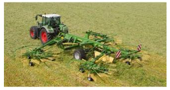
Swadro TC 1370 four-rotor centre delivery rake 10.80 m-13.70 m work widths
