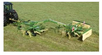
Swadro TC und TC Plus twin-rotor centre delivery rakes 5.70 m-10.00 m work widths
