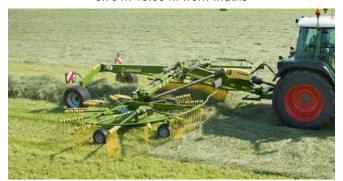
Trailed single-rotor rake 3.80 m-4.60 m work widths
