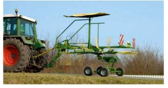
Swadro TS and TS Twin rotor side delivery rakes 6.20 m-8.20 m work widths
