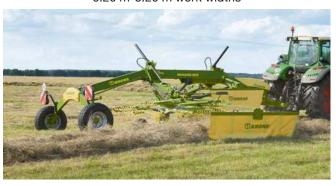
Swadro TS 970 triple-rotor side delivery rake 9.70m work width
