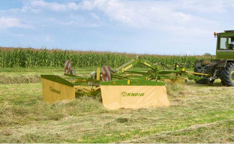
**Forming one single swath** Raking 6.20 m into one swath
