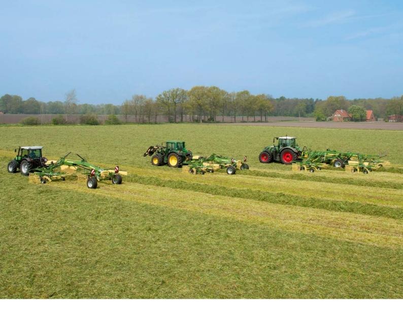
Swadro TC 1250 four-rotor centre delivery rake 9.80 m-12.50 m work widths
