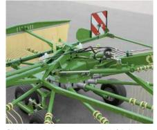
Shifting the rear rotors left/right Operators can quickly shift the rear rotor to the side by operating a ram that also varies the work width when forming one single swath.
