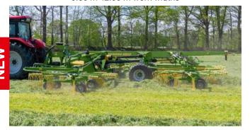
Swadro 1400 and 1400 Plus four-rotor centre delivery rakes 11.00 m-13.50 m work widths
