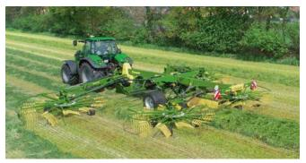
Swadro 2000 six-rotor centre delivery rake 11.00 m-19.00 m work widths
