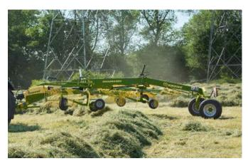
High-stability frame with a generous ground clearance Large-diameter tube steel gives the chassis and the main beam a particular strength. The high-clearance beam combines with the high-lift feature to raise the tines 50 cm (1'8") clear off the ground (may vary by model), leaving big windrows undisturbed.
