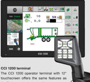
touchscreen offers the same features as the Delta terminal plus it allows operators to split the screen in two views, for example to see all machine control elements in one view and the camera footage in the other. Also, an additional AUX joystick enhances operator comfort even further.
