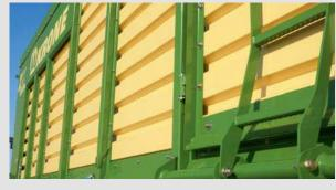
The 240 cm high stanchions are made from hat channel steel and offer ultimate durability and strength. The sides are hot-galvanized, powder-coated and plastic-laminated.Quality through and through.
