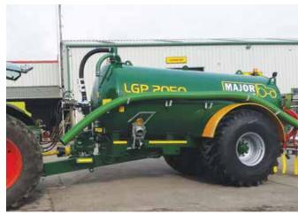
The position of the axle relative to the machine length means that a perfect balance is achieved with 80% of the weight running on the tanker's axle and the remainder being carried on the tractor drawbar.
