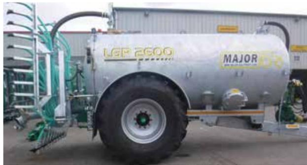
The position of the axle relative to the machine length means that a perfect balance is achieved with 80% of the weight running on the tanker's axle and the remainder being carried on the tractor drawbar.
