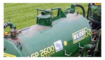
Top Fill: The hydraulically controlled top fill is used to fill the tank from the top. This option allows for high flow rates and fills the tank to its optimal level.
