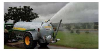
Raingun: Centre mounted or rear mounted in conjunction with a garda pump fitted with stone trap as standard.
