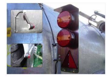
Double LED Lights: Double LED lights and LED side markers can be fitted for increased operator safety
