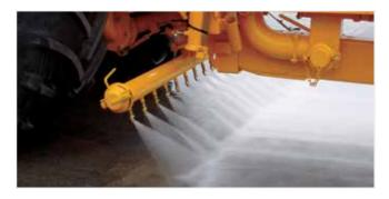
Road Blaster Unit: This unit is fitted beneath the tanker for high-pressure road washing. The angle of the nozzles can be adjusted for tough conditions
