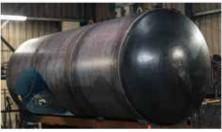
The joints on the tank are welded to ensure a high-quality and visually perfect weld seam.
