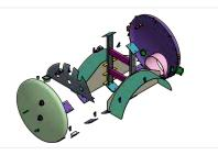
Internal baffle plates improve operator driver safety by preventing wave motions during transport.
