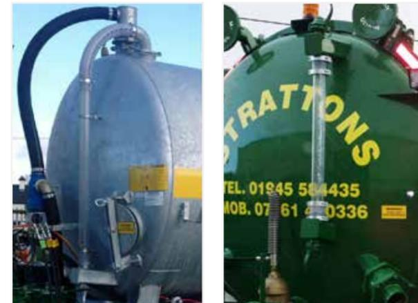
**Full Length Sight Tubes:** To allow the operator to easily identify how much liquid remains in the tank.
