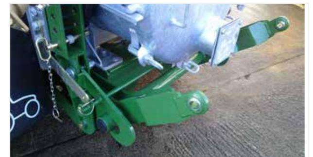
**Rear Linkages:** Linkages can be added to your tanker to allow slurry injector units to be fitted at a later stage.
