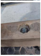
Step 4 - If you are not installing a brisket board that will fit through the mattress – use the hammer fixings and washers to secure the front.
